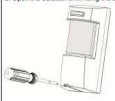
Release the detector body from the metal bracket by pulling the detector out and up.
